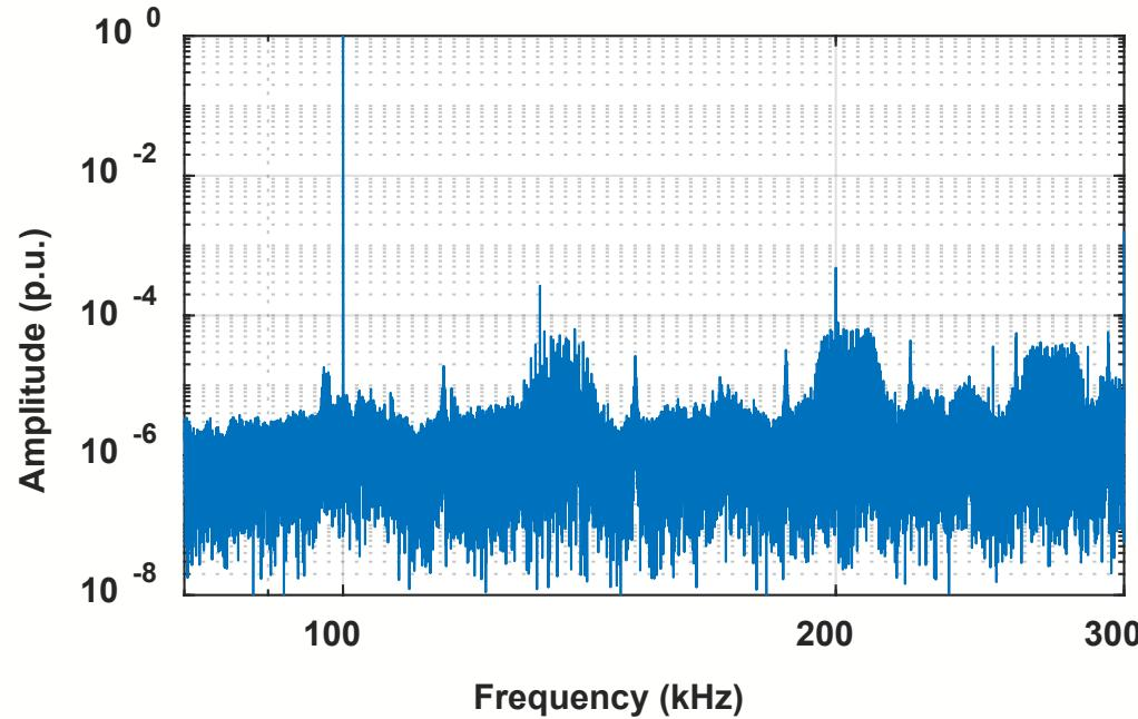
**Output spectrum ( $f_{hf} = 100 \text{ kHz}$ )**
