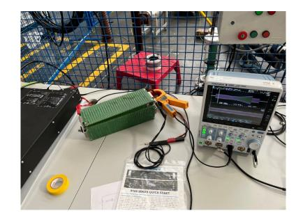
Frequency sweep characterization from 1 kHz to 150 kHz to Fluke i800s probe – Ferrite core current transformer. Constant scale factor through all frequencies.
